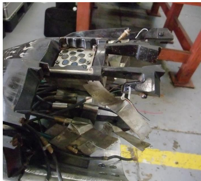
Figure 7: Damaged UT tool sensor carrier due to bore restriction
