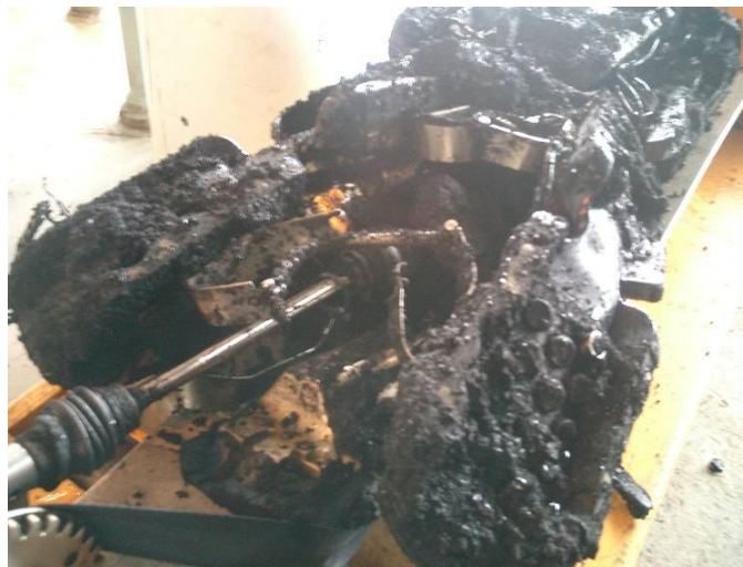
Figure 3: Damaged tool due to excessive debris
