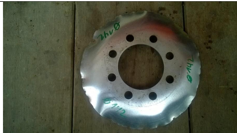
Gauge plate damage caused by weld penetrations
