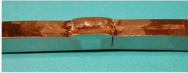
Figure 1. – HISC of Super 13Cr due to exposure to seawater with cathodic protection applied
