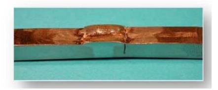
Figure 1. – HISC of Super 13Cr due to exposure to seawater with cathodic protection applied
