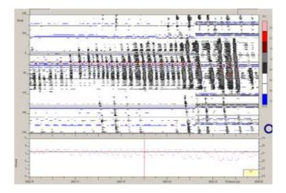
Figure 5. - Inspection results showing wrinkles in CRA liner
