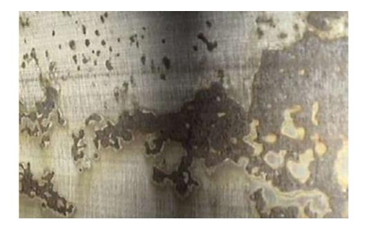
Figure 2. – Example of contamination of CRA surface of lined pipe section
