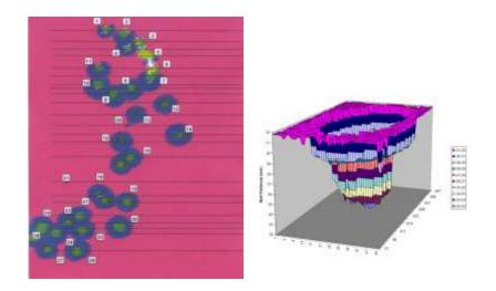
Figure 10. – Features identified during MFL inspection of carbon steel pipeline clad with 316L - Feature dimensions confirmed by external TOFD
