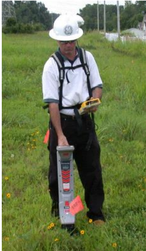
Figure 1: Locating the centreline with a pipe locator.
