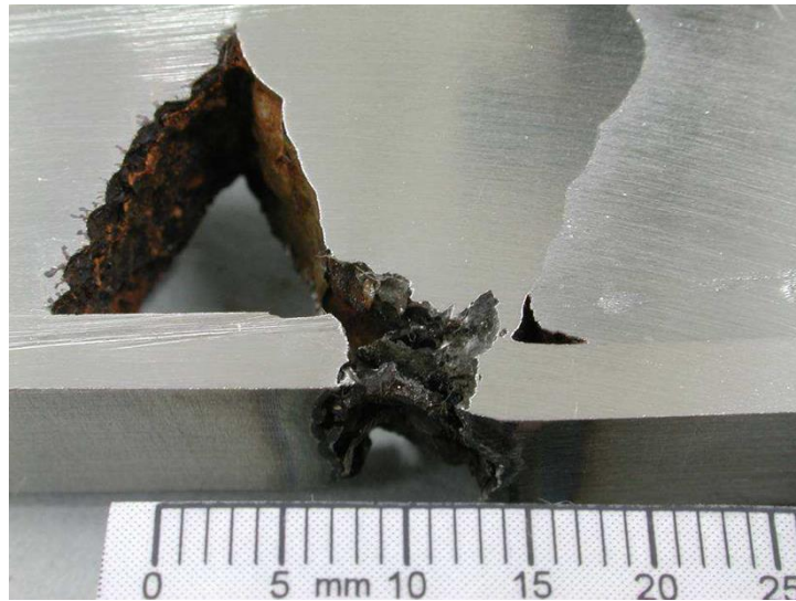
Figure 4. – Corrosion of clad pipeline due to incorrect material used for weld root
