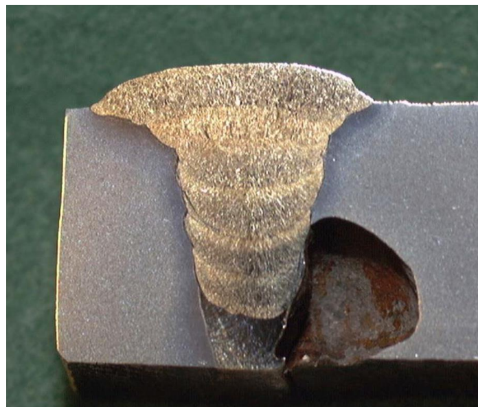
Figure 7. – Pitting of Super 13Cr due to exposure to seawater
