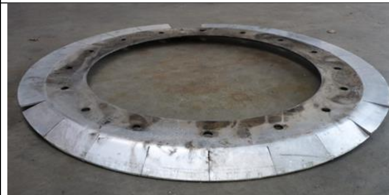
Gauge plate damaged by gate valve
