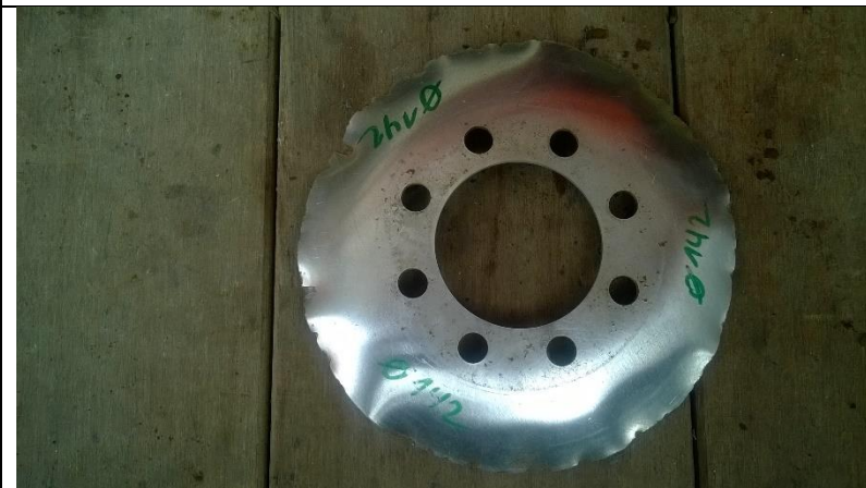
Gauge plate damage caused by weld penetrations
