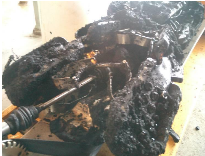
Figure 5: Damaged tool due to excessive debris
