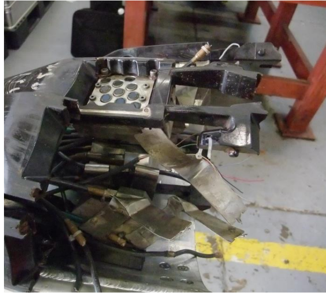
Figure 9: Damaged UT tool sensor carrier due to bore restriction
