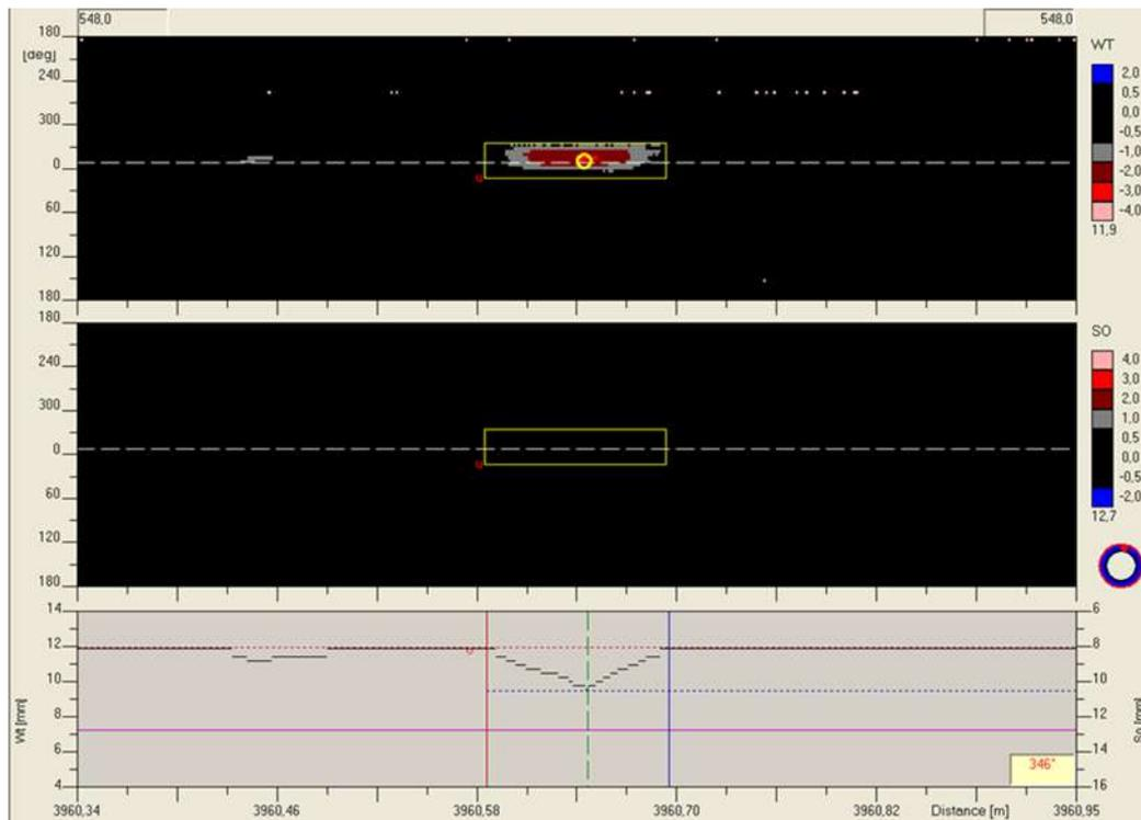
**Figure 8.** – UT ILI of external metal loss in Duplex pipe
